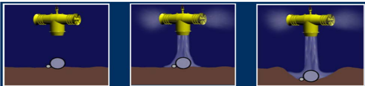
Figure 36 Mass flow excavation
