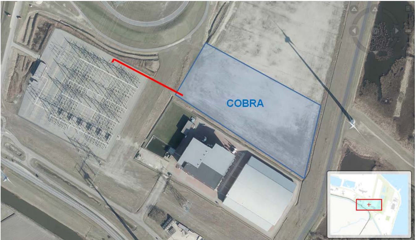
Figure 8 HVAC underground cable route (red)
