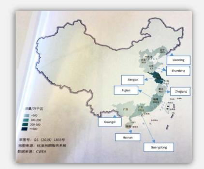
Numbers on the picture indicates the potential offshore wind capacity by per regions: capacity/10,000kilowatts
