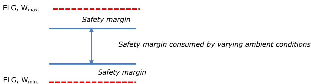
Figure 3: Schematic illustration of the safety margin consumed by varying ambient conditions
