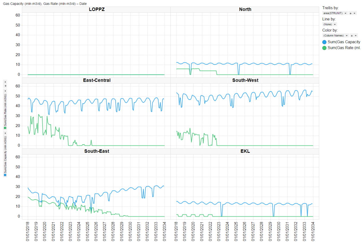
Figure 3-5: Forecasted production (green lines) and capacity (blue lines) per region for average temperature
