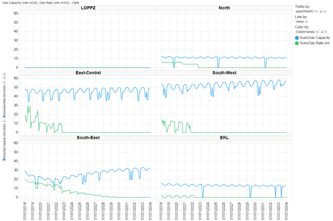
Figure 3-15: Forecasted production (green lines) and capacity (blue lines) per region for warm temperature
