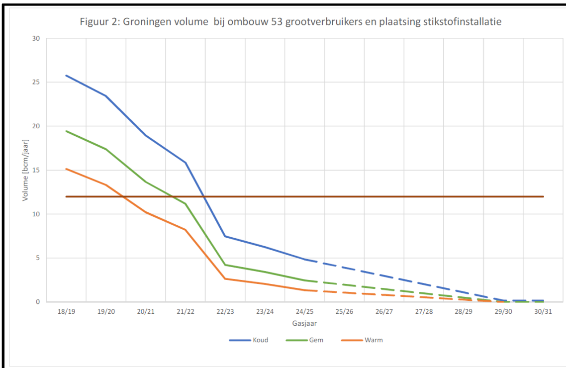
Figure 1.2 Production scenario “Basispad Kabinet” for a sequence of cold temperature years (in blue), average temperature years (in green) and of warm temperature years (in orange) from reference 7.
