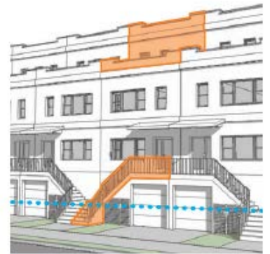
Zoning for Coastal Flood Resiliency Wider range of design options to make the streetscape more inviting while mitigating additional height
