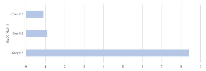
Figure 2 CO<sub>2</sub> emissions per technology<sup>13</sup>
