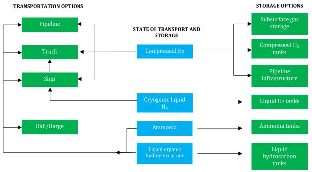
Figure 7 Main options for  $H_2$  storage and transport<sup>28</sup>
