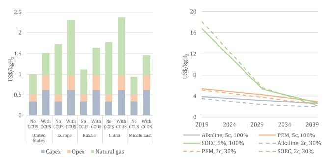
Figure 6 Hydrogen production costs using natural gas<sup>26</sup> versus hydrogen production costs using electrolysis<sup>27</sup>
