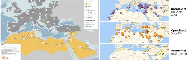
Figure 17 Simulated RE projects' locations vs. actual operational projects' location<sup>40</sup>
