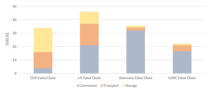
Figure 8 Global cost of energy penalty from four hydrogen value chains
