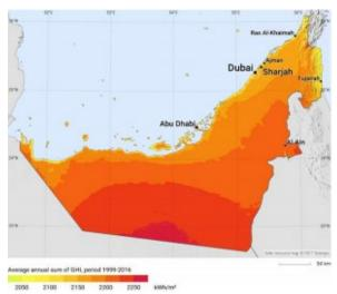
Figure 16 The UAE global horizontal irradiation
