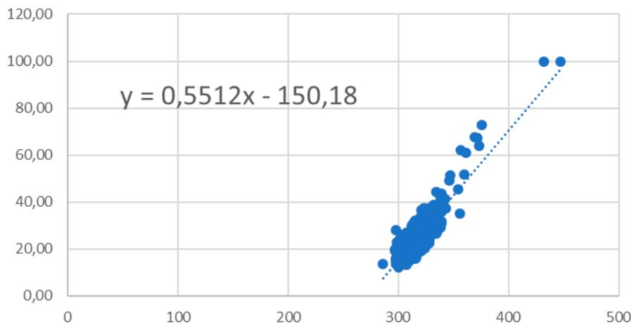
**Figure 7: server 1 CPU load vs power, high performance.** In this graph, the vertical axis shows the CPU load of the server and the horizontal axis shows the power that was measured. Each point corresponds to a measurement interval where both CPU loading and power data were collected. (for example, 20% load, 300 Watt).
