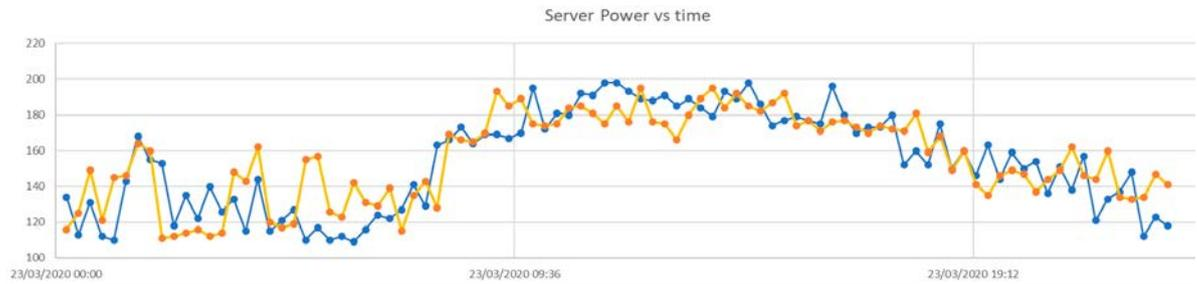
**Figure 16: Power draw of server, Blue line hardware controlled, orange line OS controlled**
