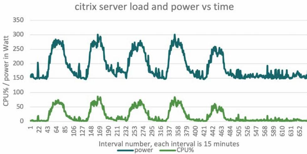
**Figure 10: Citrix server configured as “high performance”.** In this graph, the vertical axis has a double meaning. The green line shows the CPU usage as a percentage from 0% (idle) to 100% (fully loaded), the blue line shows the electrical power draw P in Watt. The horizontal axis just shows the number of the measurement interval.
