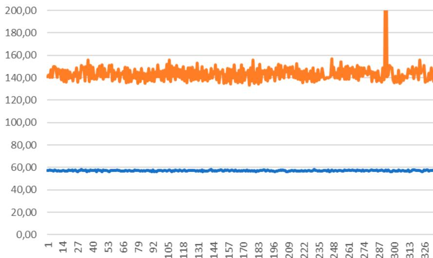
**Figure 9: single server configured with “favor performance”.** In this graph, the vertical axis has a double meaning. The blue line shows the CPU Idle as a percentage from 0% (fully loaded) to 100% (idle), the orange line shows the electrical power draw P in Watt. The horizontal axis just shows the number of the measurement interval.
