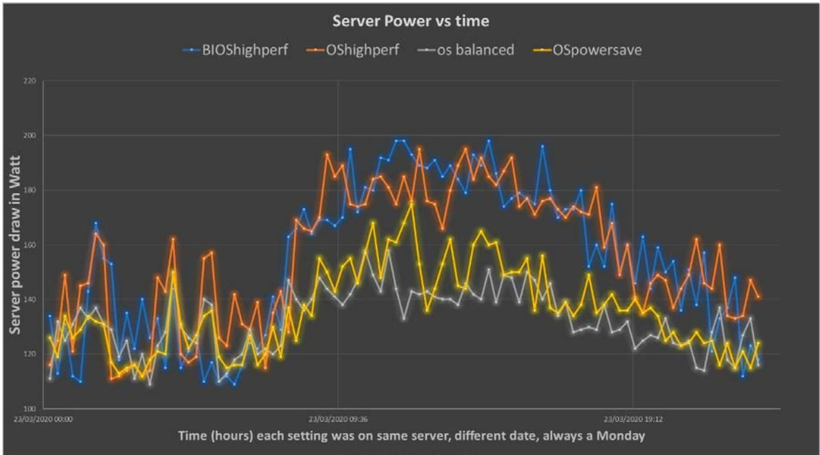
**Figure 18: Measurements including “power save” mode**
