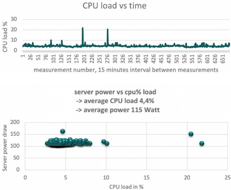
**Figure 12: underloaded server configured as “static high performance”.**
