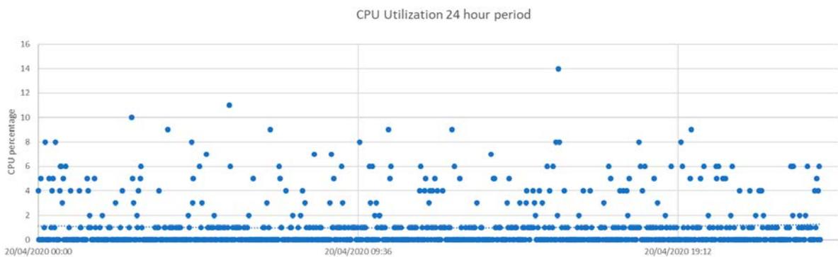
**Figure 15: 24 hours recording of CPU usage**
