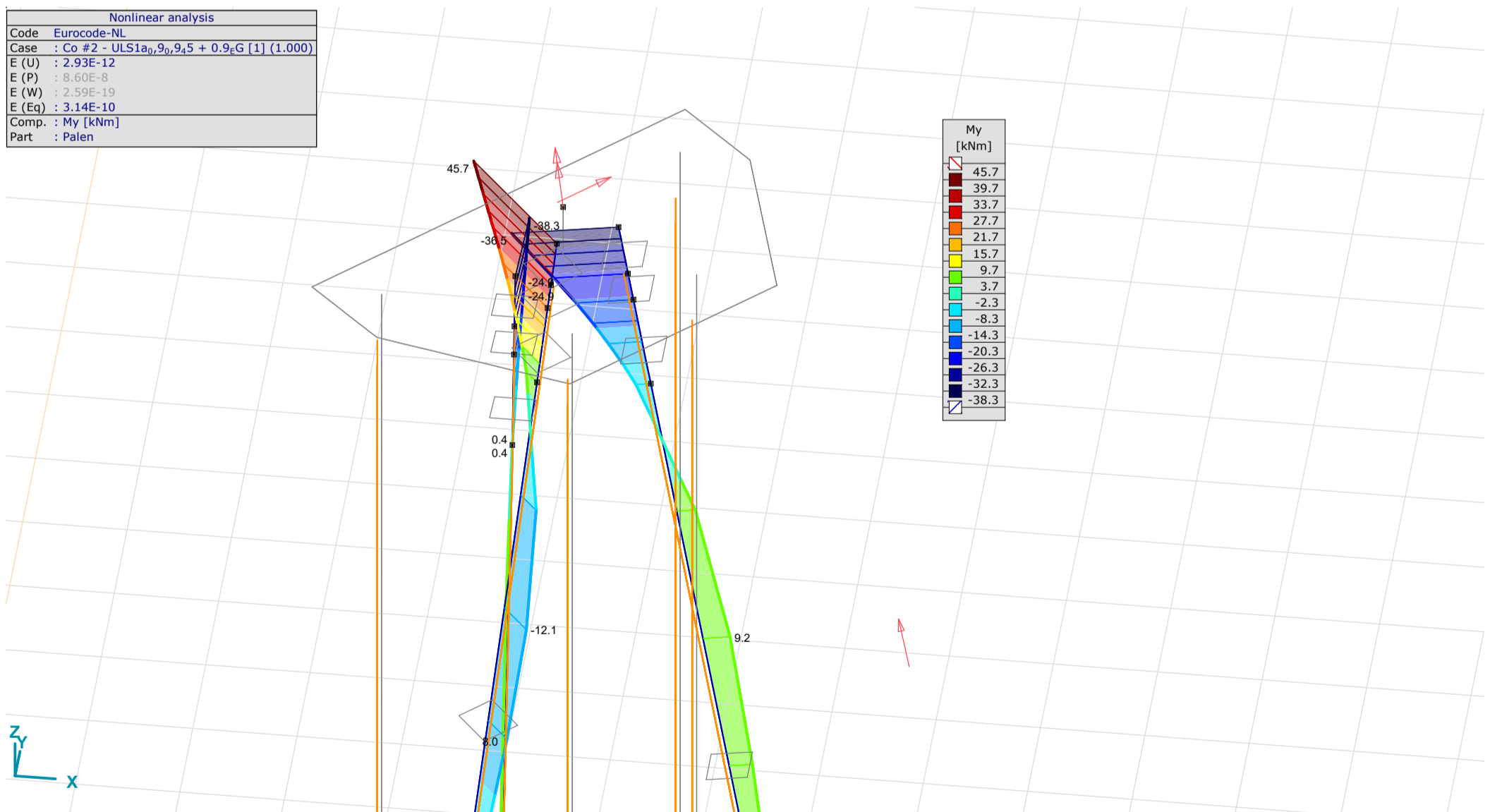
old Piles, Nonlin., Co # 2 - ULS1a_0,9_0,9_45 + 0.9_EG [1] (1.000), My, Filled diagram
