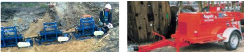
Figure 18 Typical cable tensioners (left) & cable winch (right)
