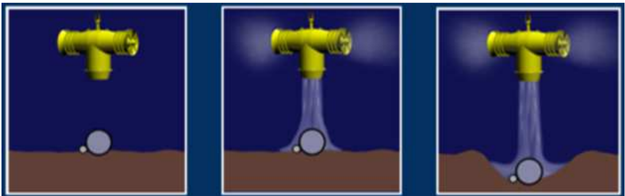
Figure 43 Mass flow excavation
