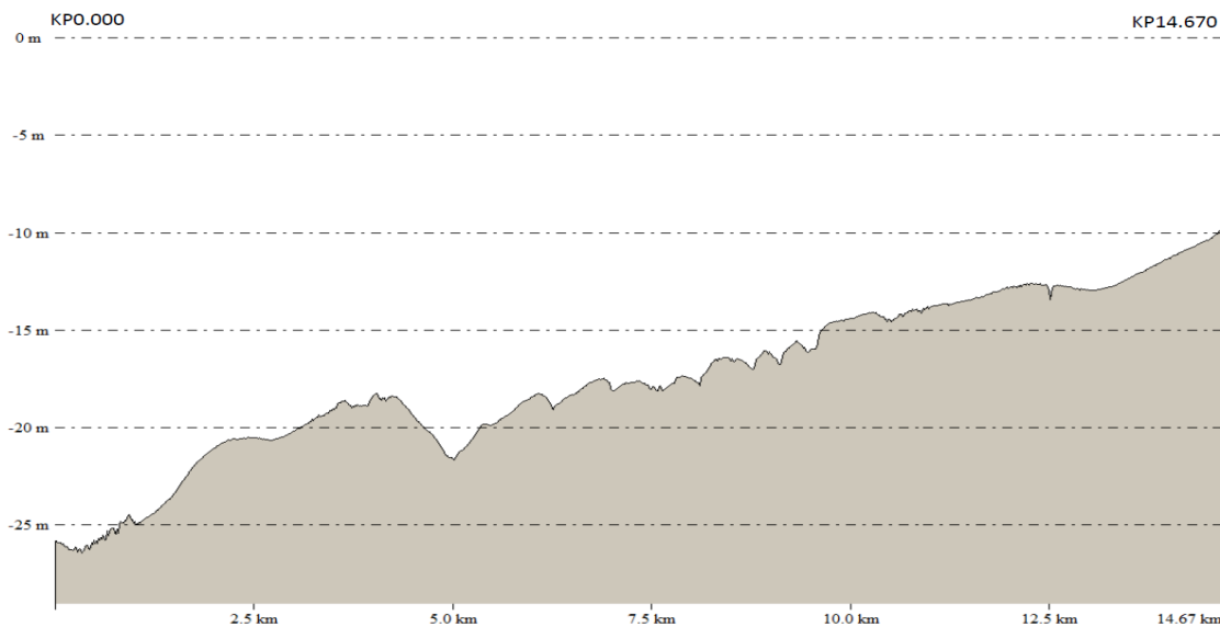
Figure 4-3 Seabed profile along pipeline route from P11-Unity Platform to Wye
