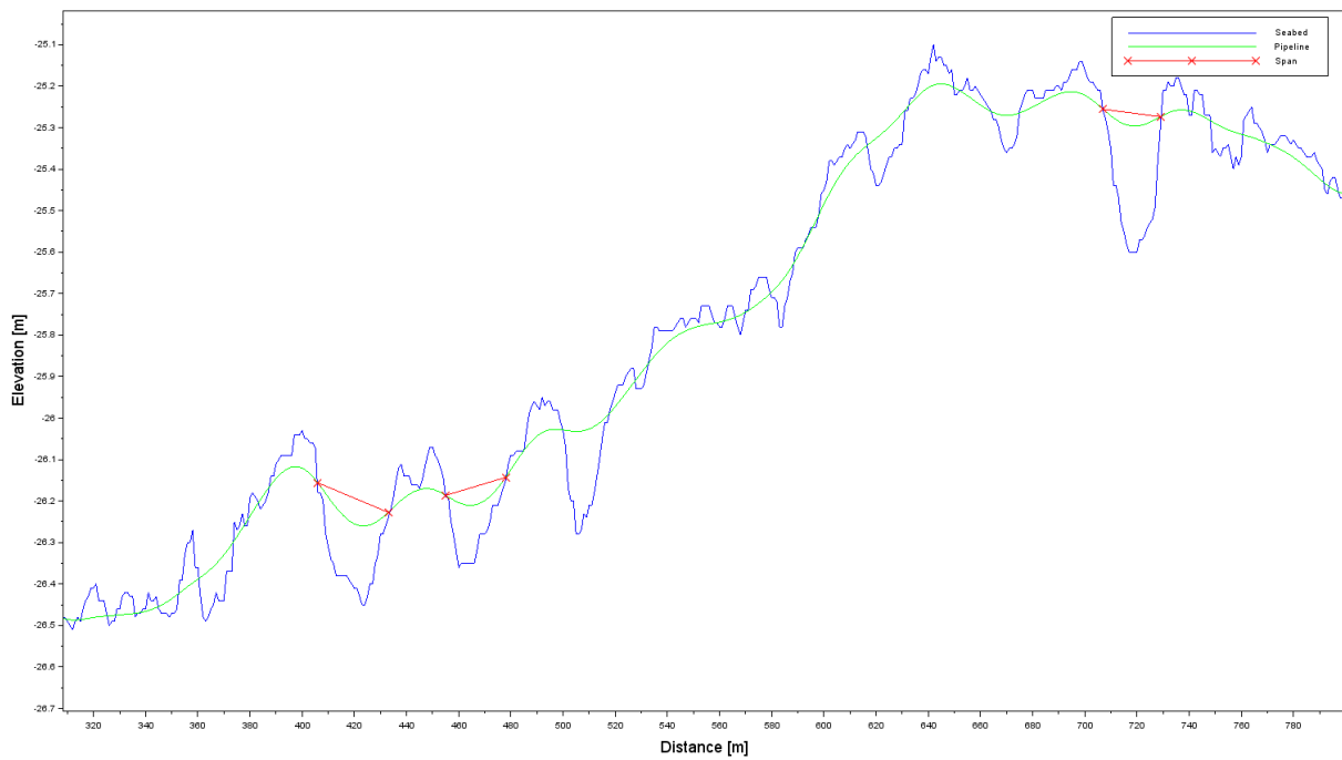
Figure 8-3 Pipeline on sea floor – section with spans >20m
