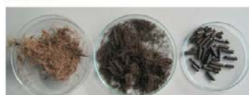
Empty fruit bunches (EFB, shredded), before and after Torwash®, and after pelletization
