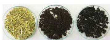
Arundo donax, before and after Torwash®, and after subsequent pelletization
