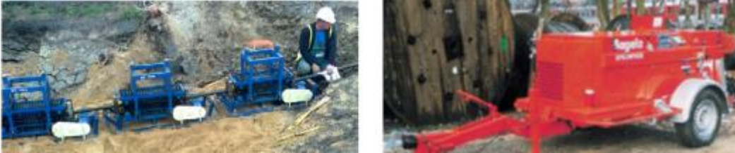
Figure 18 Typical cable tensioners (left) & cable winch (right)
