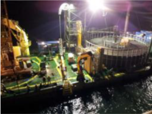
Figure 48 Typical nearshore cable lay barges
