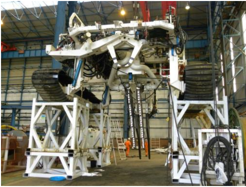
Figure 42 Typical ROV Jet trencher
