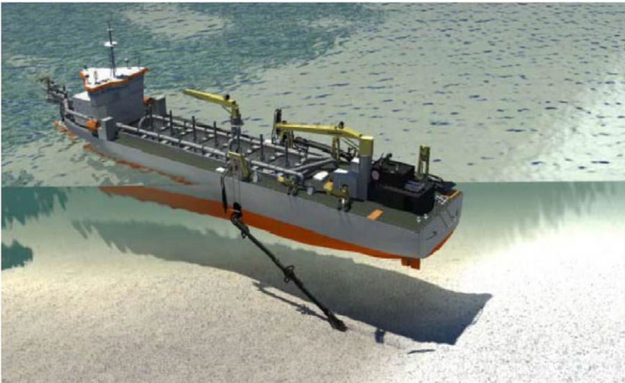
Figure 55 Trailing Suction Hopper Dredger
