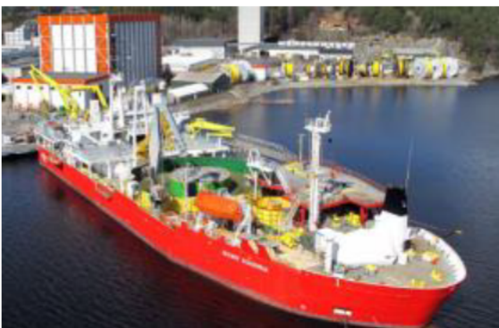
Figure 38 Typical deep water cable installation vessels
