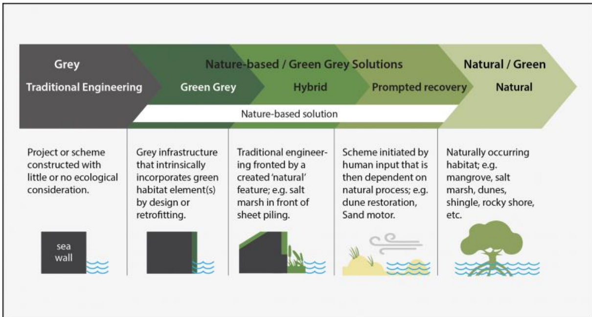
Figure 1 – Engineering solutions can be grey or green or somewhere in between. The spectrum from grey to green is continuous (Source: University of Glasgow, https://oppla.eu/product/19909 ).
