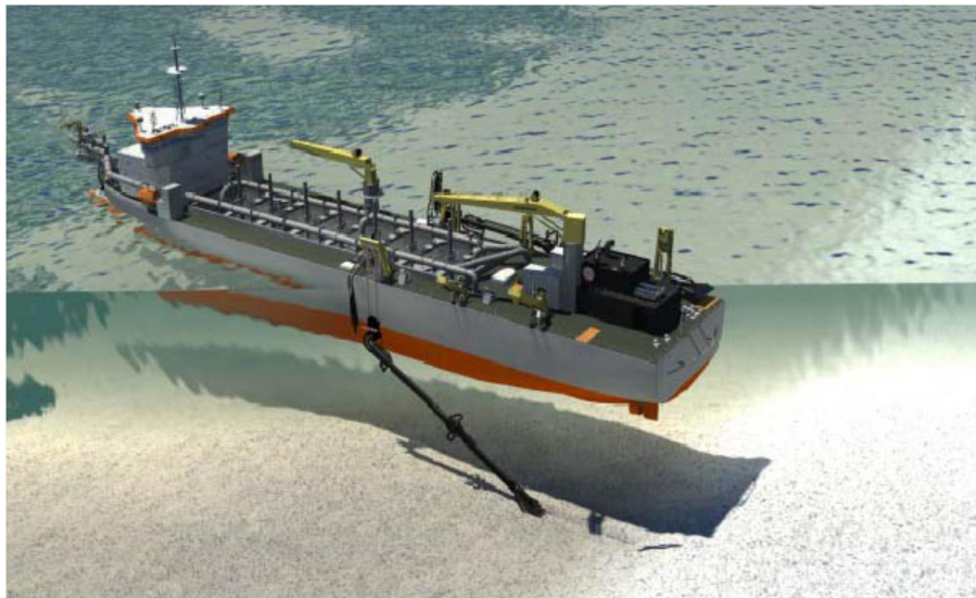
Figure 18 Trailing Suction Hopper Dredger
