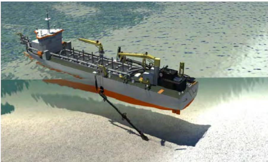
**Figure 18 Trailing Suction Hopper Dredger**
