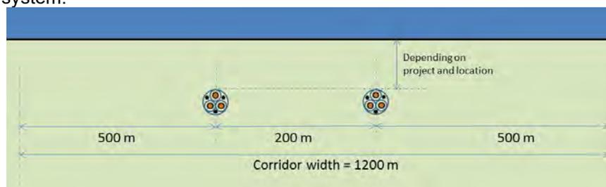
**Figure 17 - layout of 700MW export cable system**
