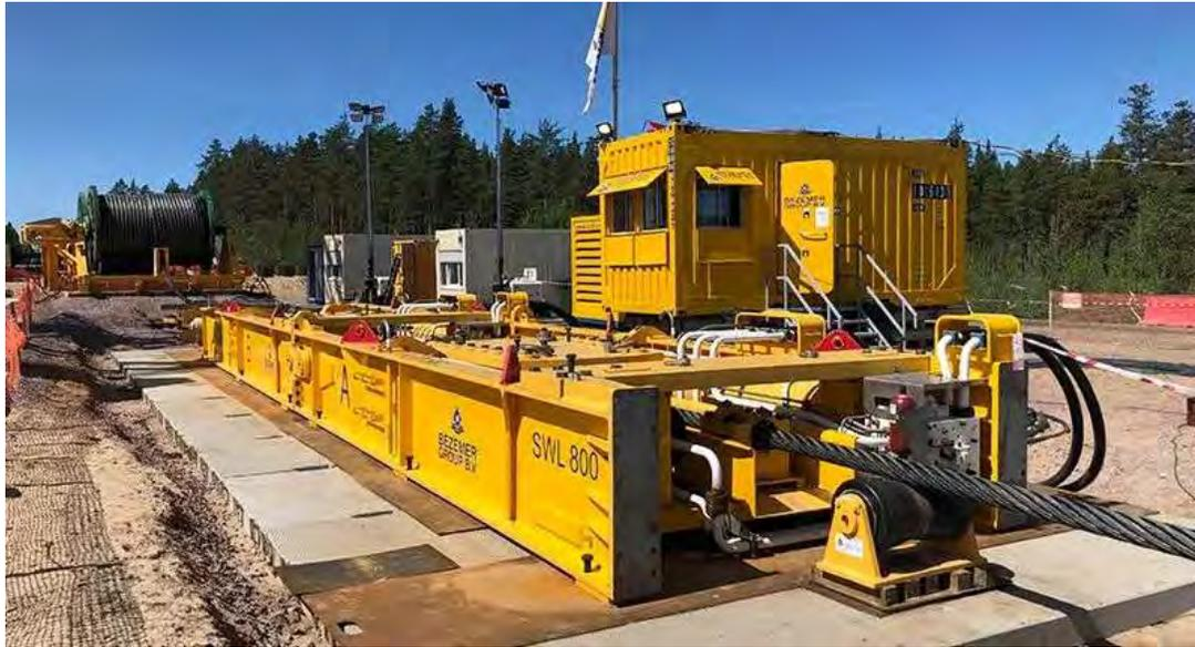
Figuur 2-15 Bezemer 800 ton lier ([https://bezemer.com/products/linear-winches/](https://bezemer.com/products/linear-winch/))
