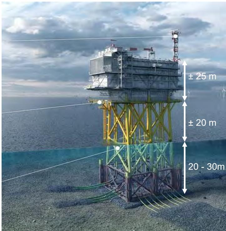
**Figure 5 Standardized 700 MW AC offshore substation concept**
