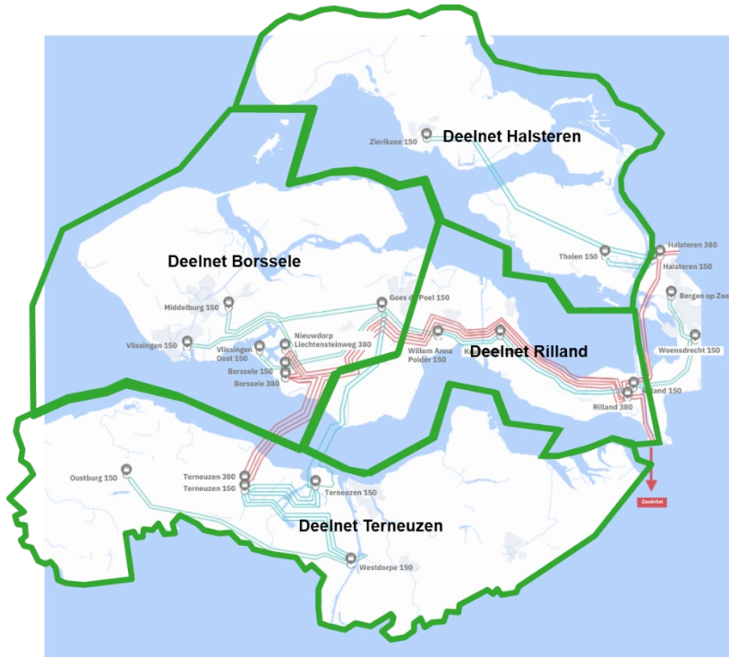
Figure 1: Subdivision of the HV grid in the province Zeeland into four 150 kV pockets.
