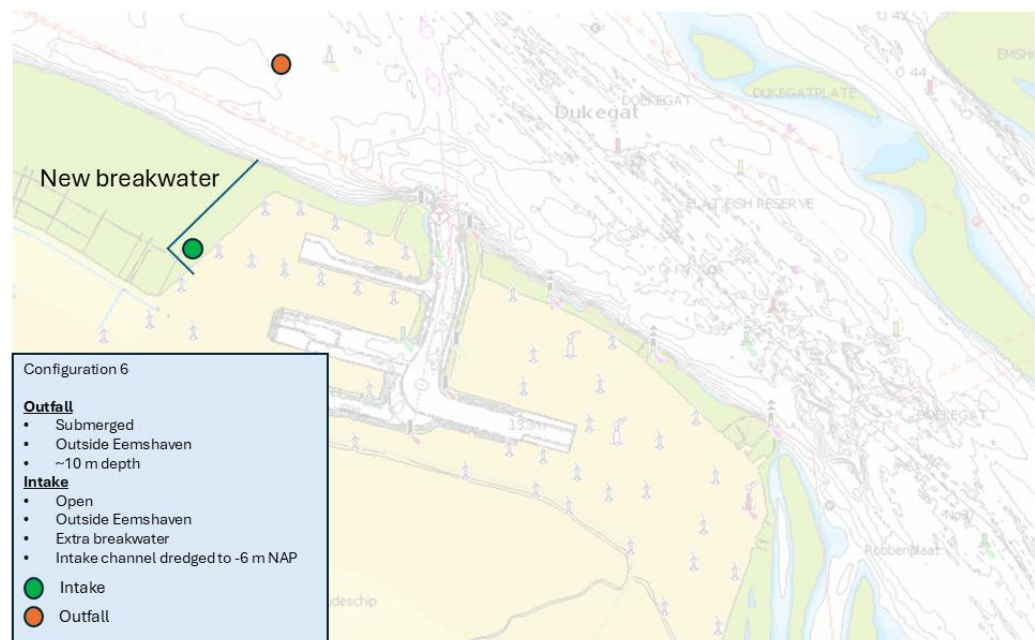
Figure 2.12 Eemshaven NPP intake and outfall Configuration 6.
