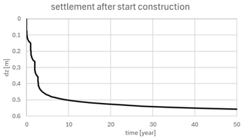
Figure 7.6 Settlement-as function of time at foundation level ( z = \text{NAP} - 7 \text{ m} ), Site 2. t = 0 years represents the start of the preparation of the site.
