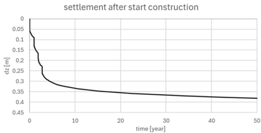
Figure 7.5 Settlement-as function of time at foundation level ( z = \text{NAP} - 7 \text{ m} ), Site 1. t = 0 years represents the start of the preparation of the site.
