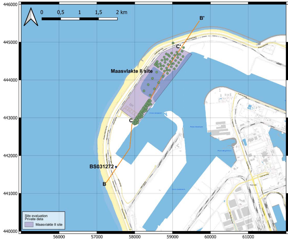
Figure 6-2 The cross section line and the location of the used CPT's relative to the cross section.
