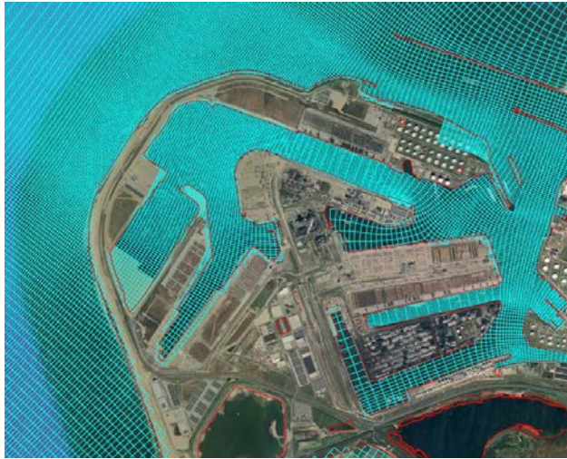
Figure 3-5 Zoomed in plot of the computational grid of the detailed Delft3D-FLOW model near project site area.
