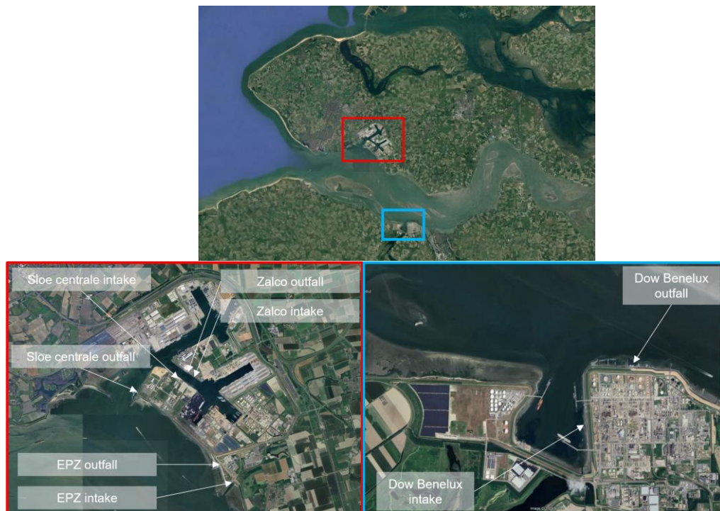
Figure 2-5 Overview existing intakes and outfalls in the project area.
