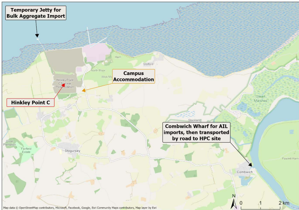
Figure 12: Sea transport infrastructure and on-site accommodation campus (HPC)
