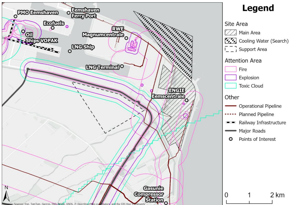
Figure 14: Attention areas, Eemshaven 3
