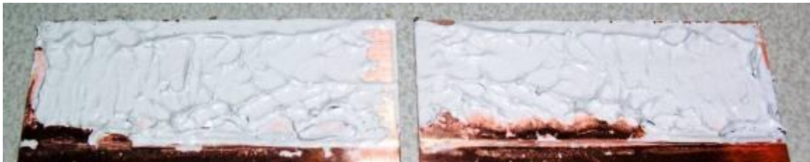
Figure 30: DC 3-6655 silicone after the adhesion test.
