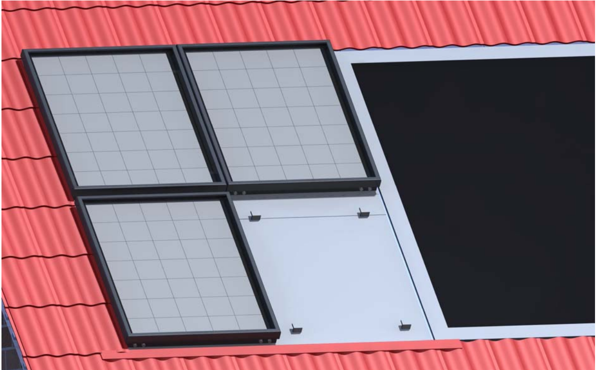
Figure 85: Panels placed next to a dormer
